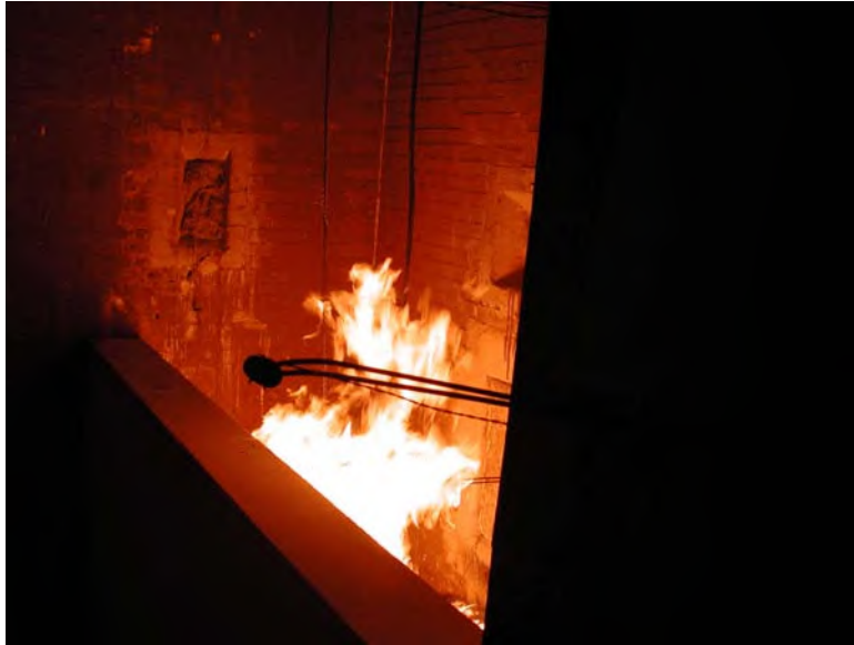
Figure 19 Photograph of Pool Fire in Trench
