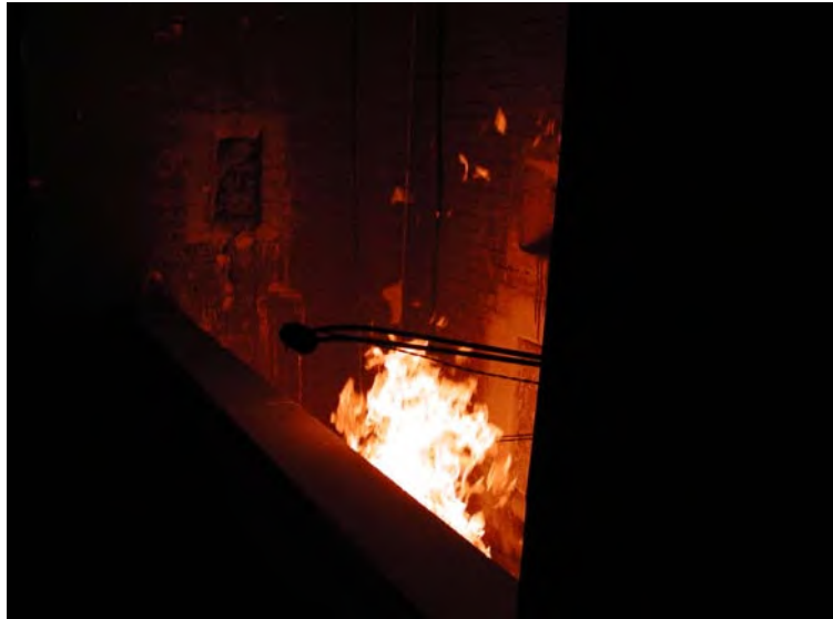
Figure 17 Photograph of Pool Fire in Trench
