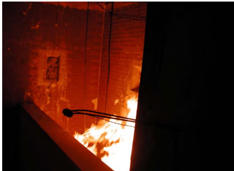
Figure 20 Photograph of Pool Fire in Trench
