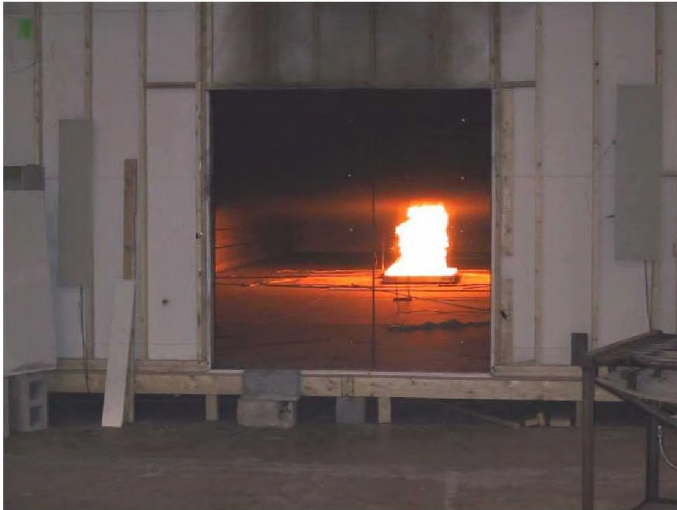
Figure 3.3 Hot Gas Layer in Test 3
