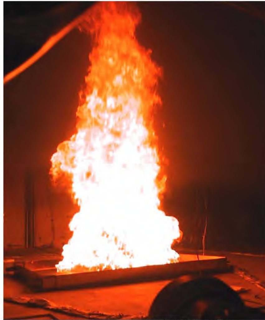
Figure 3.9 Partially Under Ventilated Fire in Test 13 (2 MW)
