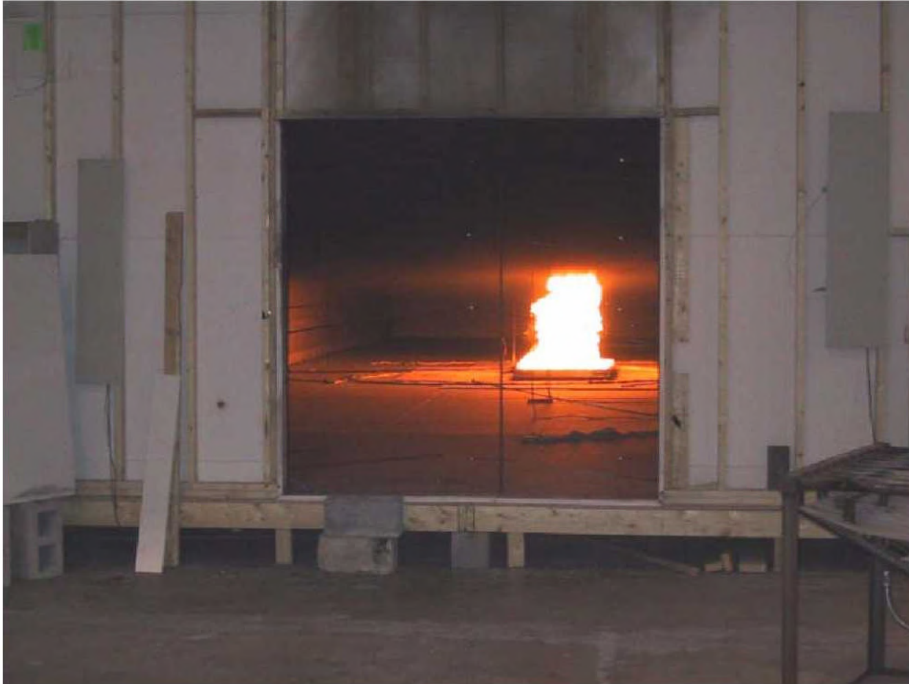
Figure 3.3 Hot Gas Layer in Test 3
