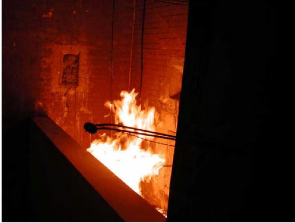
Figure 2-11 Pool Fire in Trench in Benchmark Exercise No. 5
