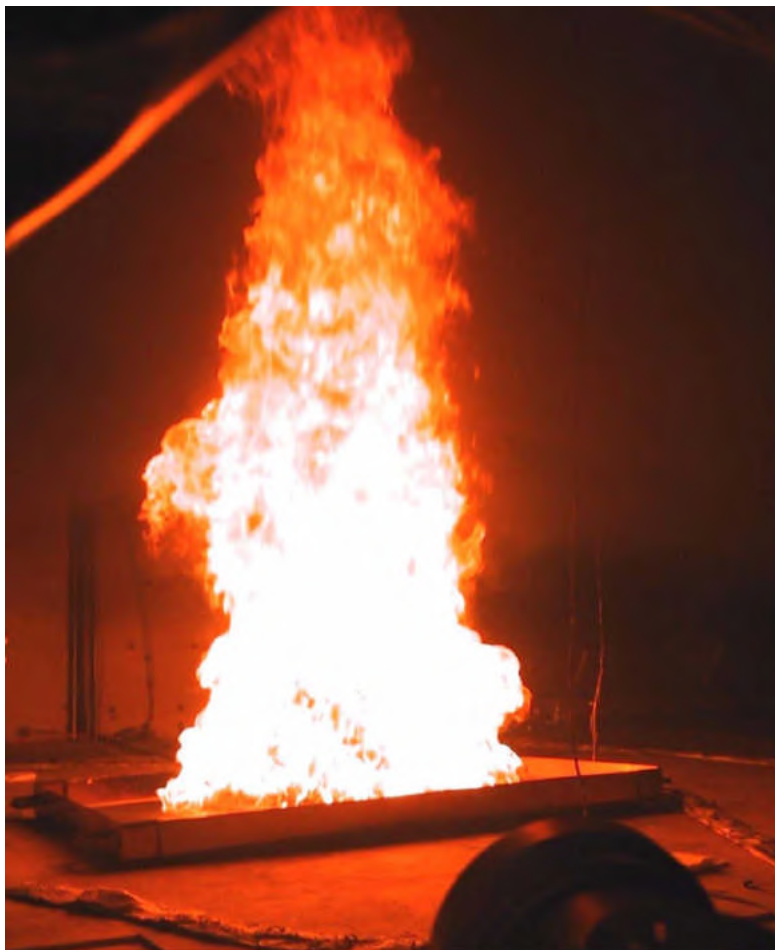
Figure 2-6 Under-Ventilated Fire in Test 13 of Benchmark Exercise No. 3
