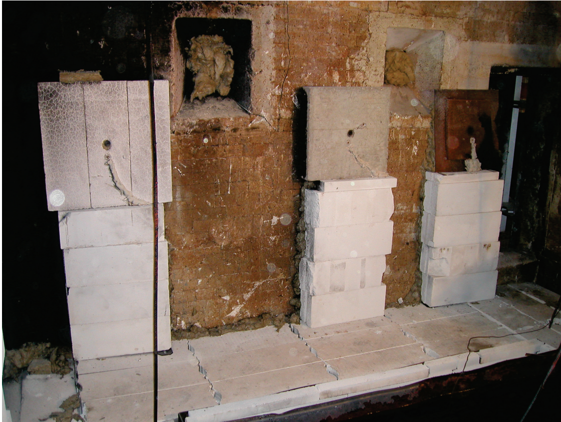
Fig. 2-20 View of the three material probes implemented in the Benchmark Exercise No. 4 test compartment
