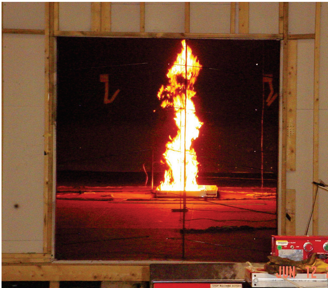
Fig. 2-15 Photograph of a Benchmark Exercise No. 3 experiment conducted in a large compartment at NIST
